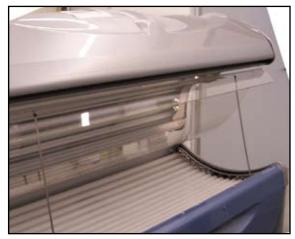
4. Remove the tube covers on the right-hand and left-hand side. To do so, take hold of the tube cover with both hands close to the edge, pull straight towards the centre of the sunbed, and take it out in an upward movement. Make sure that you pull out the lateral parts of the cover completely without canting them.
