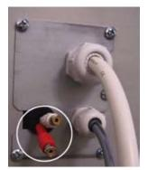
The cinch marked in the illustration is connected to the external audio source where the line-out of the sound player or the headphone/loudspeaker jack are available for connection.
