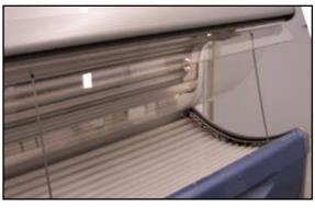
4. Pull out the front cover in upward direction and towards the front.
