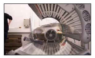
5. Remove the tube cover from the facial area. To do so, take hold of the tube cover with both hands close to the edge, pull straight towards the centre of the sunbed, and then take it out in a downward movement. Make sure that you pull out the lateral parts of the cover completely without canting them.
