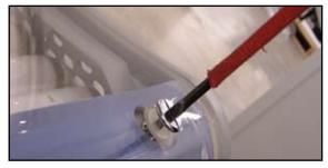
3. Lift the pane so that you are able to take out one of the pane holders located behind the front edge. Lift the pane further and erect the pane holder beyond the resistance point so that the rod stays in the fitting. Repeat this procedure for the second pane holder so that the pane rests on both holders.
