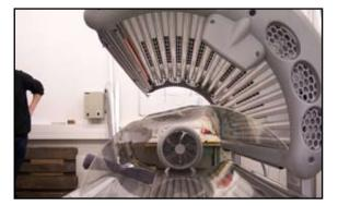
5. Clean the inner surface of the canopy pane and re-fasten it. The quick-release fasteners of the pane are screwed down as follows: Bring the screw slot into a horizontal position with a screwdriver and press against it until the lock catches.
