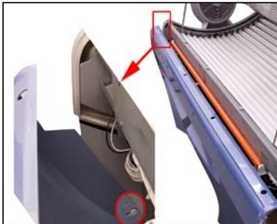
5. Pinch the coloured jacket and loosen the tube by turning it a quarter. Pull it out and replace the starter.
