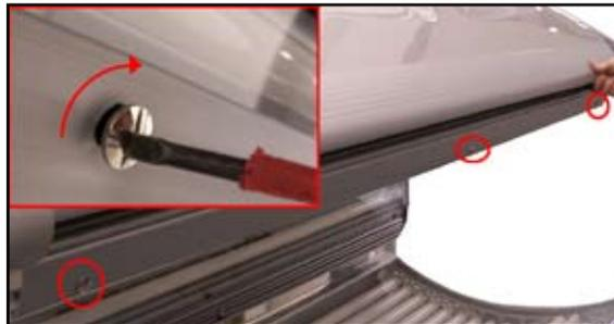
3. Take hold of the canopy pane in the front area from underneath and push it slightly towards the back side of the sunbed to release it from the holder.
