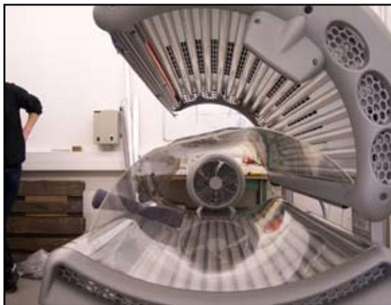
4. Remove the tube covers on the right-hand and left-hand side. To do so, take hold of the tube cover with both hands close to the edge, pull straight towards the centre of the sunbed, and take it out in a downward movement. Make sure that you pull out the lateral parts of the cover completely without canting them.
