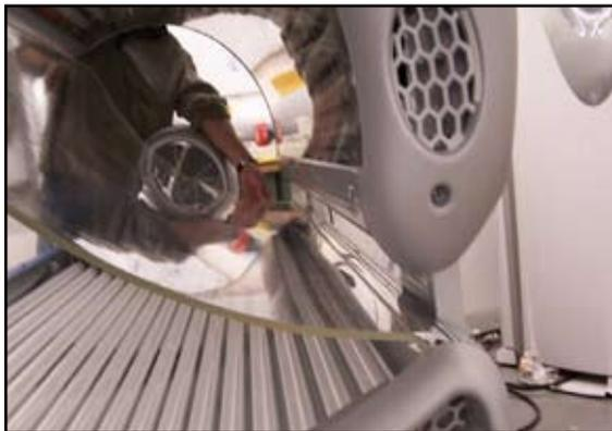
4. Assembly is performed in reverse order. Ensure the correct placement of the pane profile in the hinge profile when inserting the new pane.
