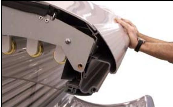
5. Pull the gas spring off the lower bolt.
