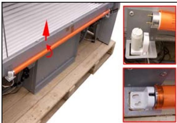
6. Insert the new tube into the jacket. Install the new tube in the fitting.
