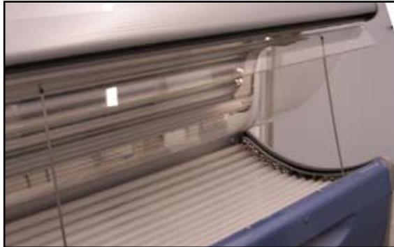
4. Pull out the front cover in upward direction and towards the front.
