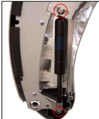
4. Take the load off the canopy by having the second person lift it somewhat and hold it in this position. The canopy may not be strained until the new gas spring has been installed with bolts and lock washers.
