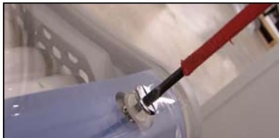
3. Lift the pane so that you are able to take out one of the pane holders located behind the front side. Lift the pane further and erect the pane holder beyond the resistance point so that the rod stays in the fitting. Repeat this procedure for the second pane holder so that the pane rests on both holders.
