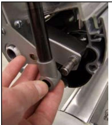
6. Draw the bolt of the upper fitting backwards and pull out the gas spring downwards.
