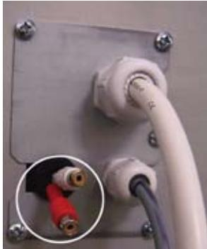
The cinch marked in the illustration is connected to the external audio source where the line-out of the sound player or the headphone/loudspeaker jack are available for connection.
